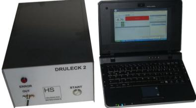
The Druleck 2 tests balloons and catheters via gas pressure. The easy and fast handling from the Druleck 2 makes a 100 % inspection possible. The Druleck has two freely programmable pressure thresholds. The first pressure threshold messures the diameter from the balloons and the second makes the maximum pressure test. The pressure is also freely programmable and goes up to 30 bar.
